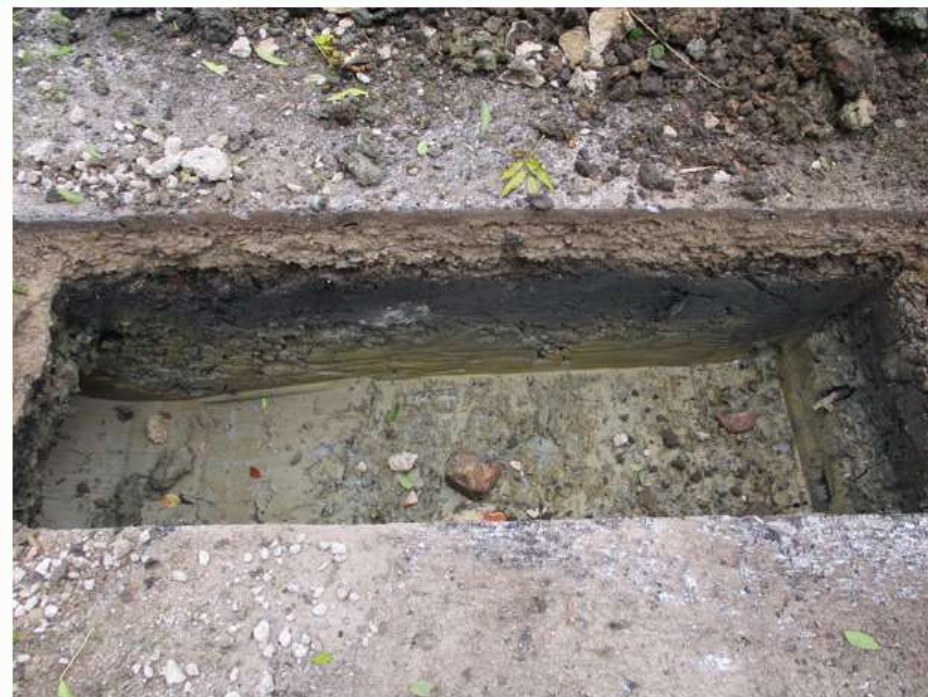
Photo No.4: TP02 pit sides and base (excavated through tarmac and concrete base)
