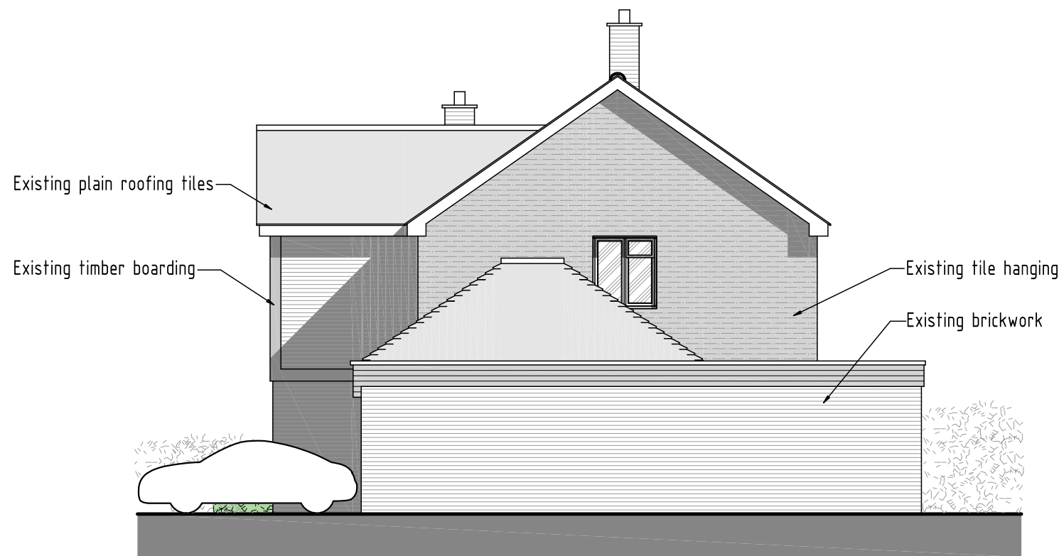
EXISTING SIDE ELEVATION - 1:100
