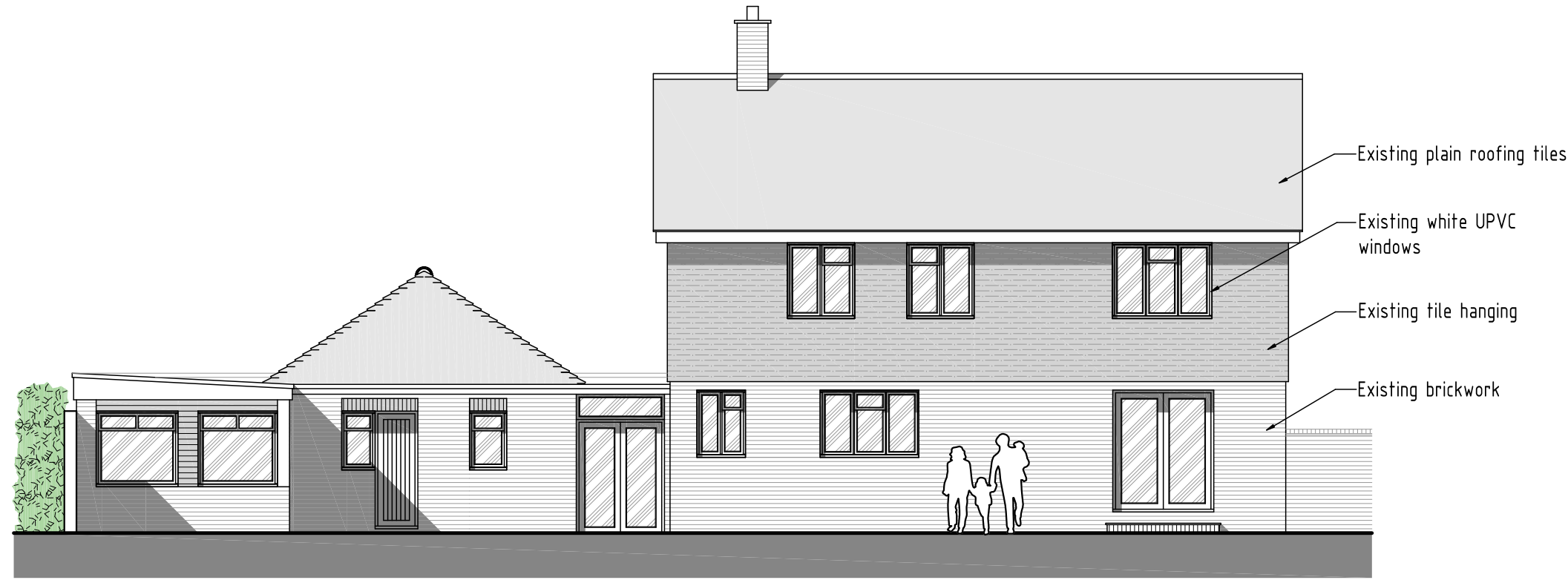
EXISTING REAR ELEVATION - 1:100
