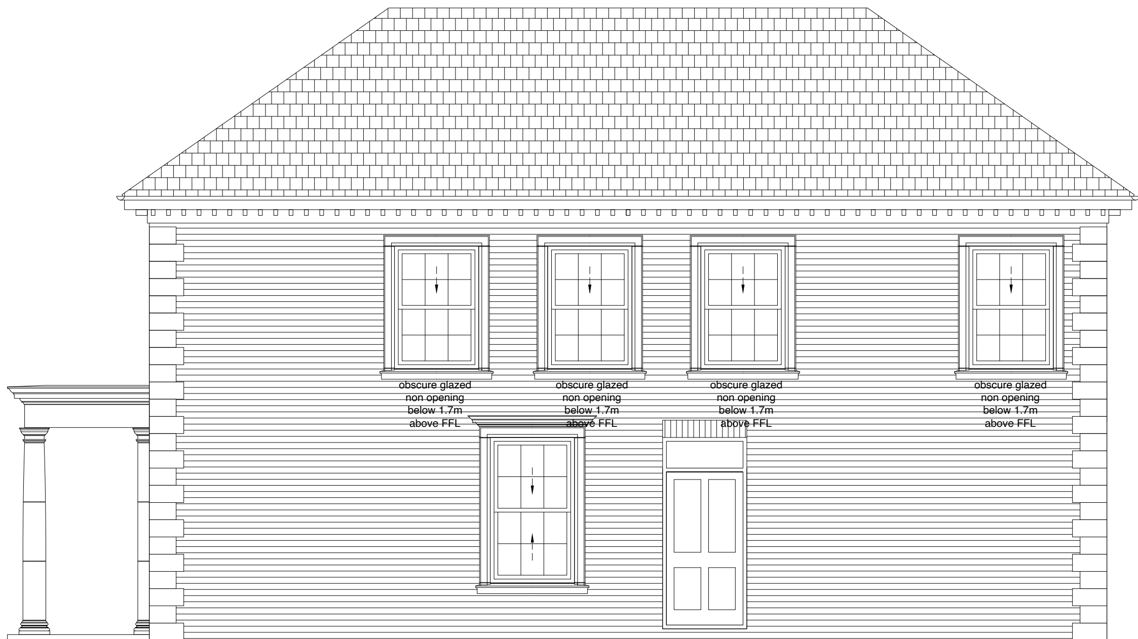
PROPOSED FLANK ELEVATION
