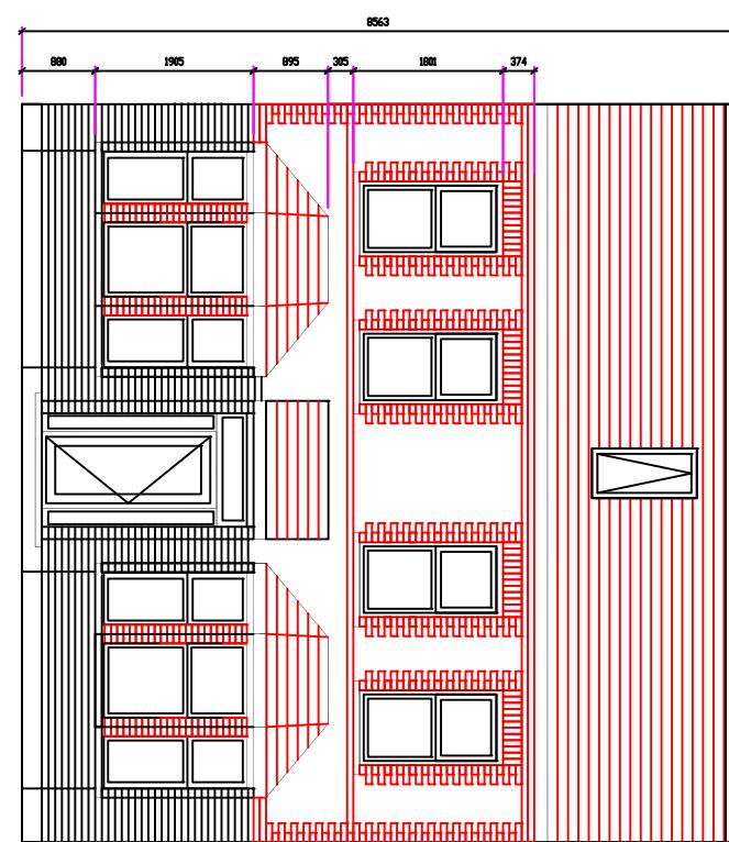
Features of new building to match adjacent building in Levels and style with contrasting materials to match existing
