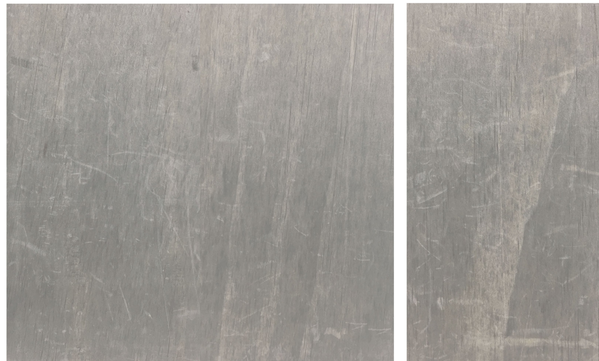
2. TIMBER Accoya or similar modified softwood naturally weathered to silver grey colour
