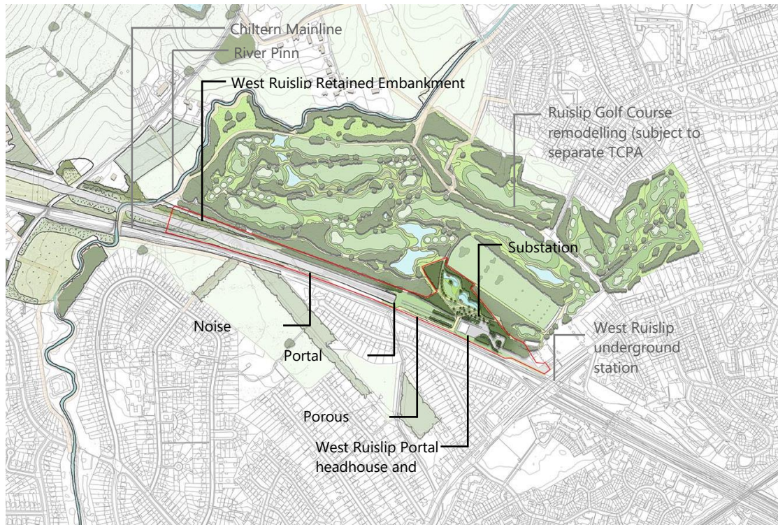
Figure 7 - Schematic plan of the main elements within the application boundary and surrounding area
