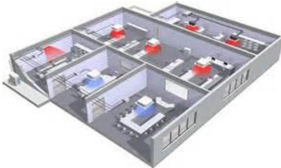
Fig.3 - Typical VRF heating and cooling system
