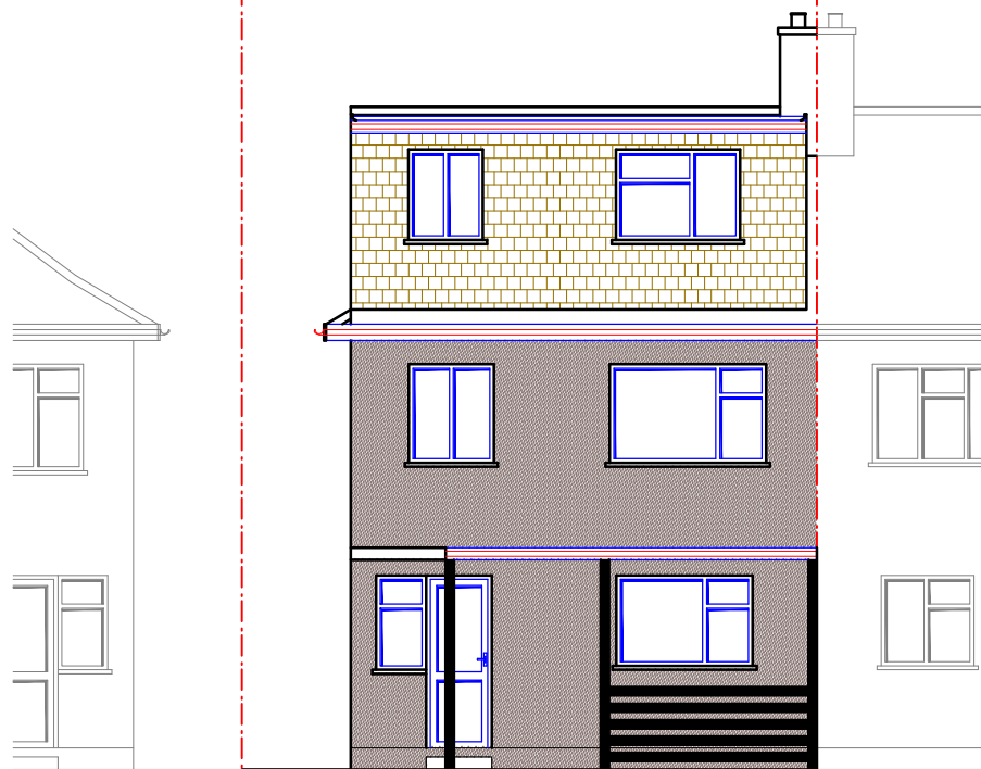
EXISTING REAR ELEVATION
