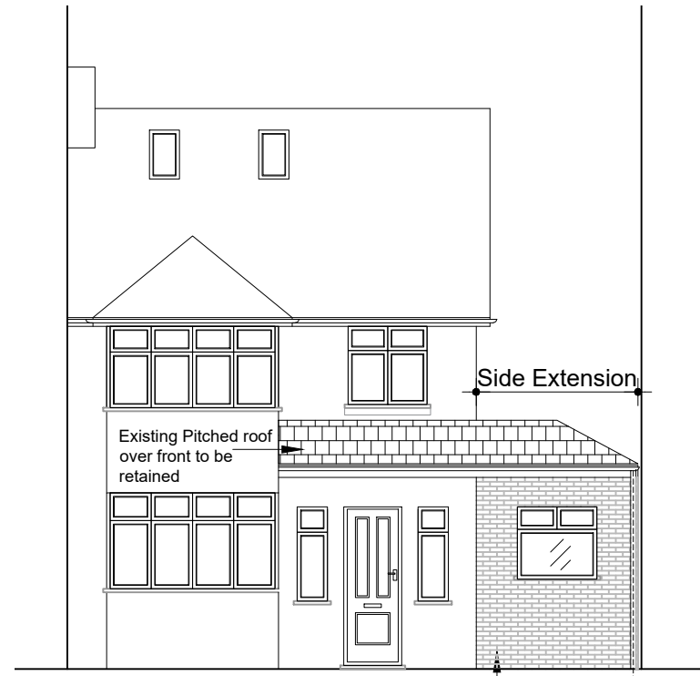
Front Elevation Showing Proposed Side Extension- Sc 1:100
