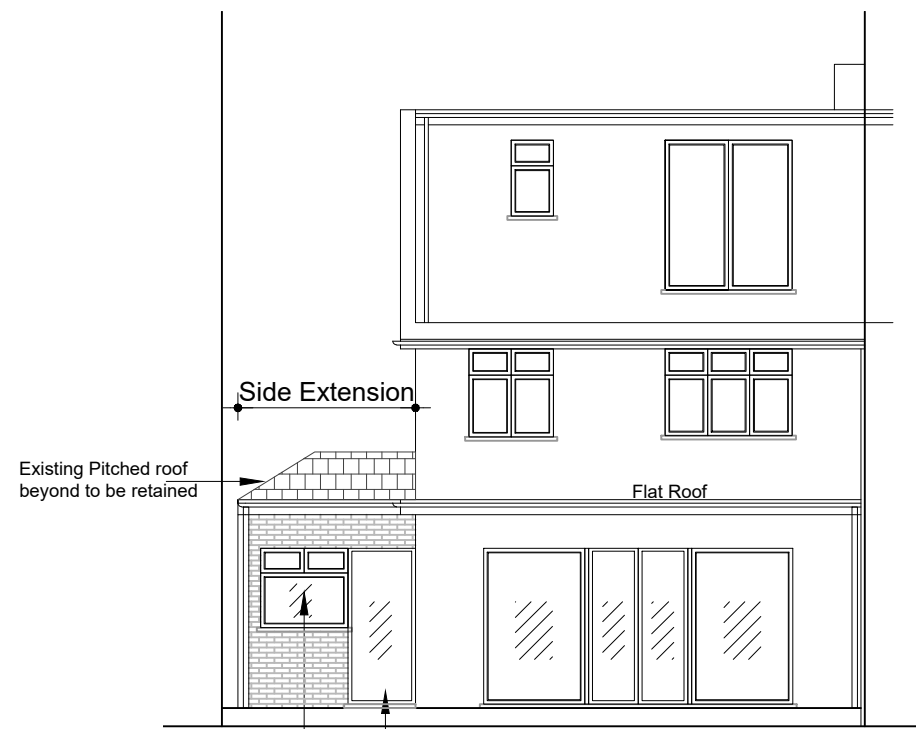
Rear Elevation Showing Proposed Side Extension- Sc 1:100
