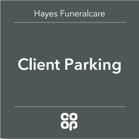
Item 5 3No. parking Sign. 3mm aluminium folded panel. Panel to be powder coated RAL 7010 and fixed with 25x25x3mm angle. Vinyl text. Size: 600mm x 600mm Scale: 1:10
