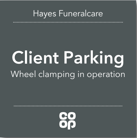
Item 4 2No. Parking Sign. 3mm aluminium folded panel. Panel to be powder coated RAL 7010 and fixed with 25x25x3mm angle. Vinyl text. Size: 600mm x 600mm Scale: 1:10
