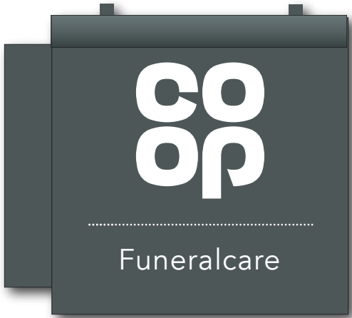
Item 3 1No. Externally illuminated Projector sign. RAL 7010 with white applied vinyl lettering. Consisting of 2mm folded aluminium panels having 50mm returns fitted back to back around steel support framework, with mild steel projecting arms and fixing plate, being powder coated RAL 7010. Size: 550mx550mm Scale: 1:10
