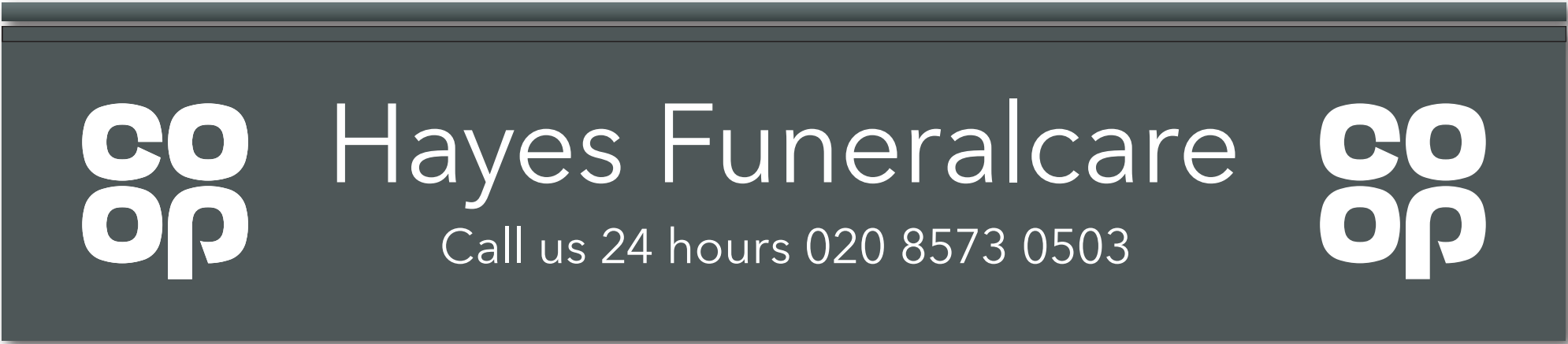
Item 1 1No. Externally illuminated fascia with applied vinyl lettering and Co-op logo. Fascia to be powder coated RAL 7010, lettering to be white. Size: 5250mm x 1055mm (including 50mm upstand) 50mm returns. Scale: 1:20
