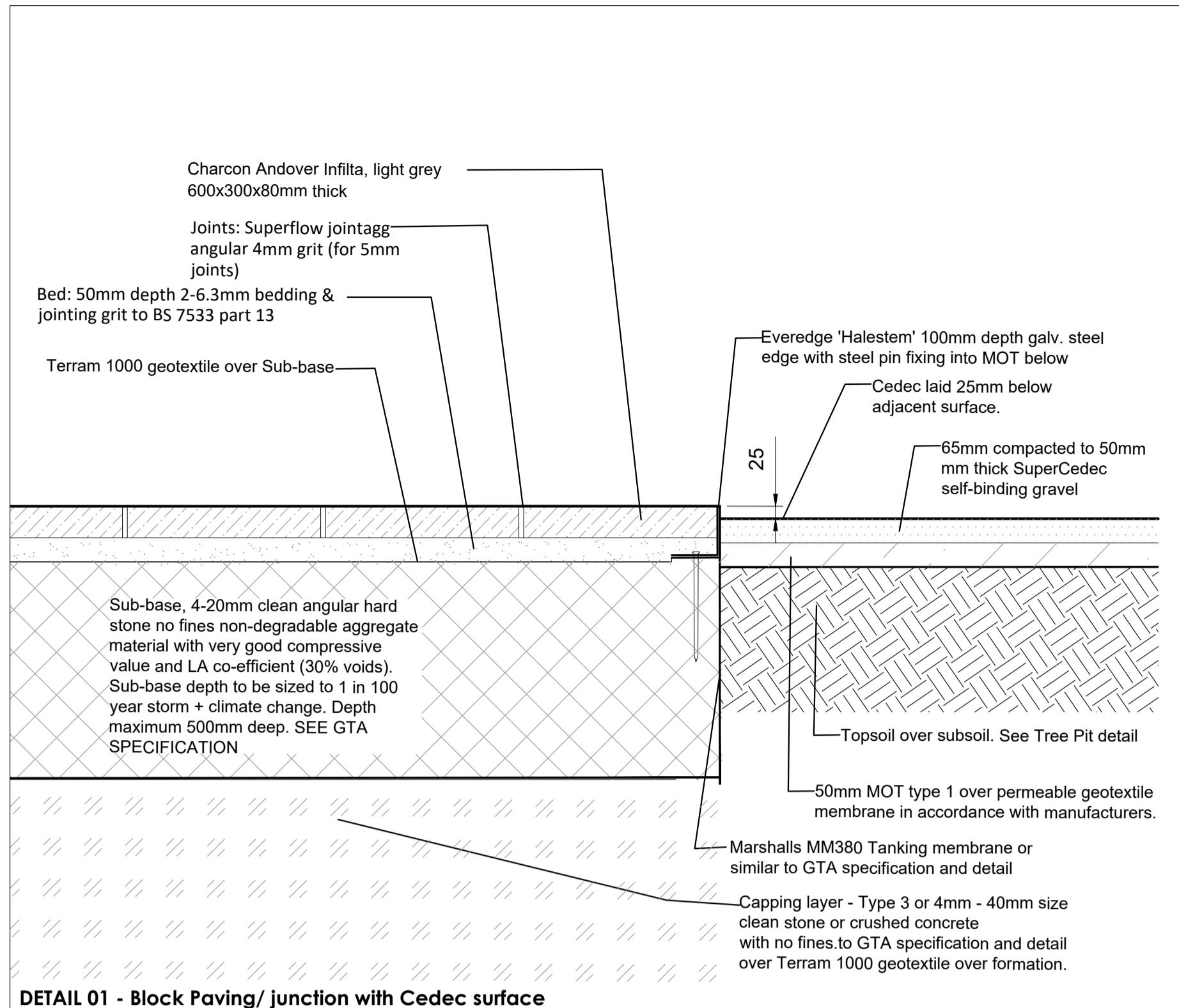
**DETAIL 01 - Block Paving/ junction with Cedec surface**
