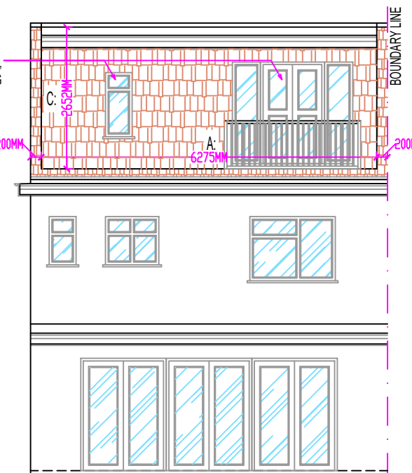
PROPOSED REAR ELEVATION SCALE 1:100@A1
