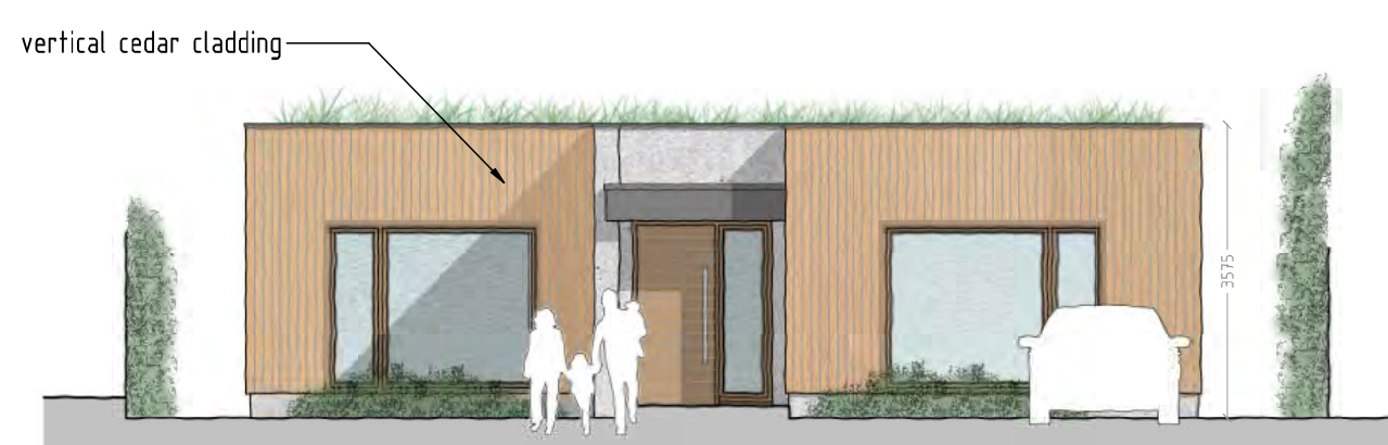
FRONT ELEVATION SCALE 1:100
