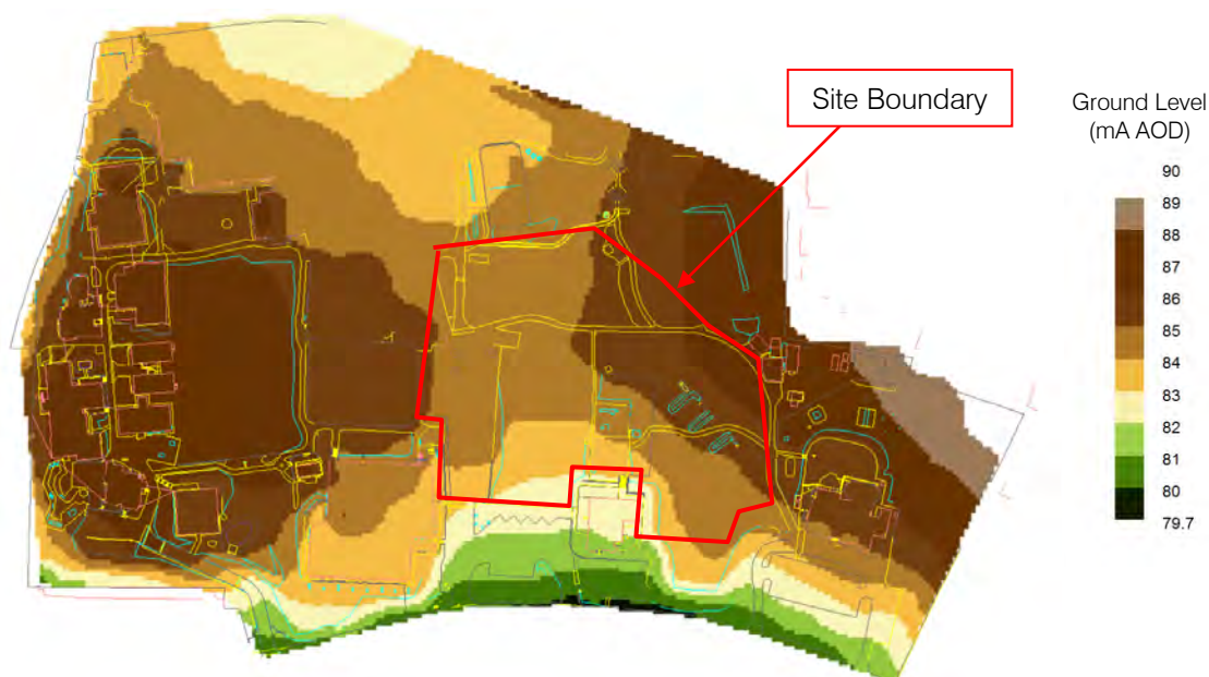
Figure 2 – Ground Model Produced from Topographical Survey
