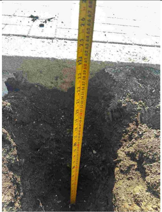
600mm thickness example within Block E (Ground Level)
