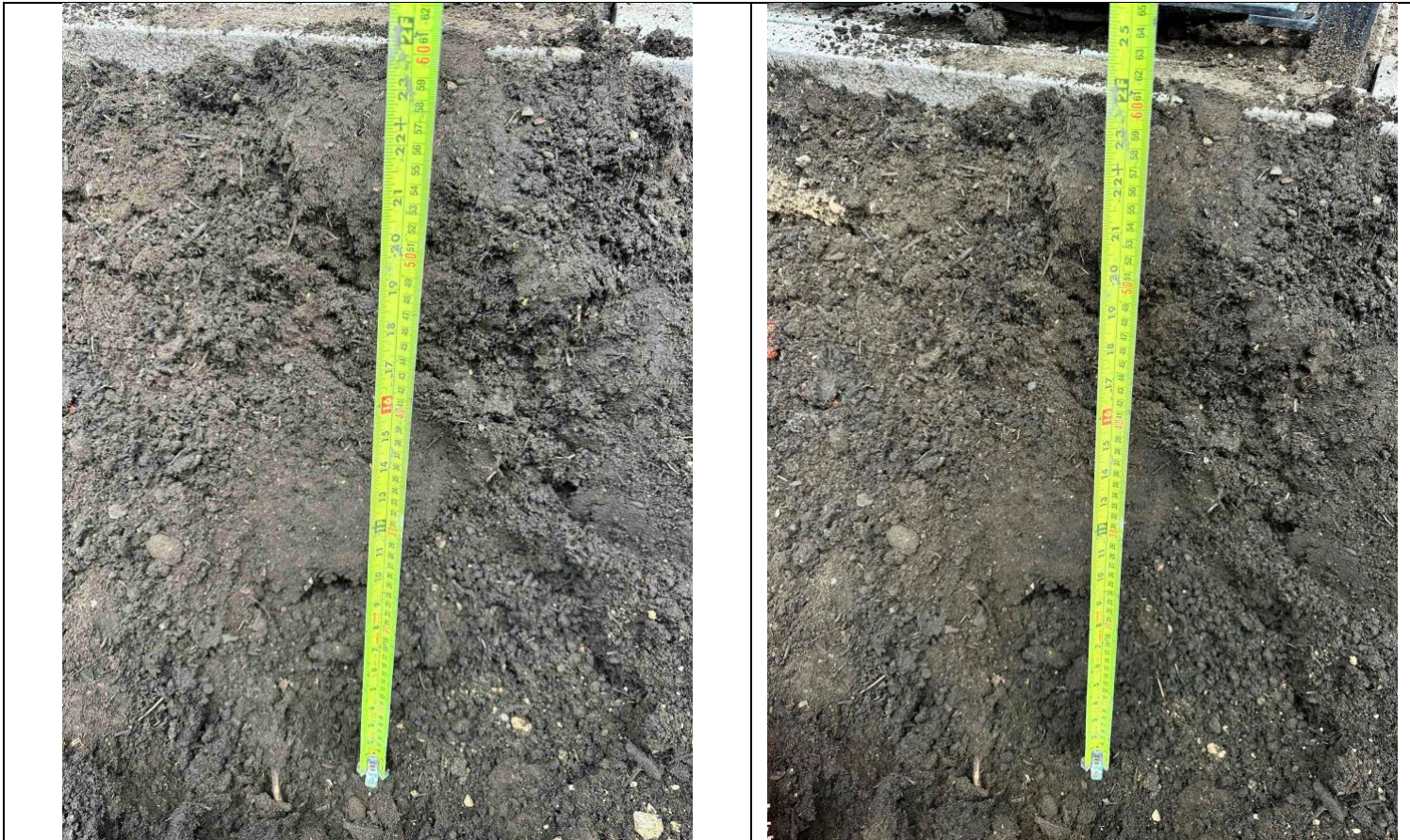
Example of 60cm topsoil thickness (Blocks A and D)
