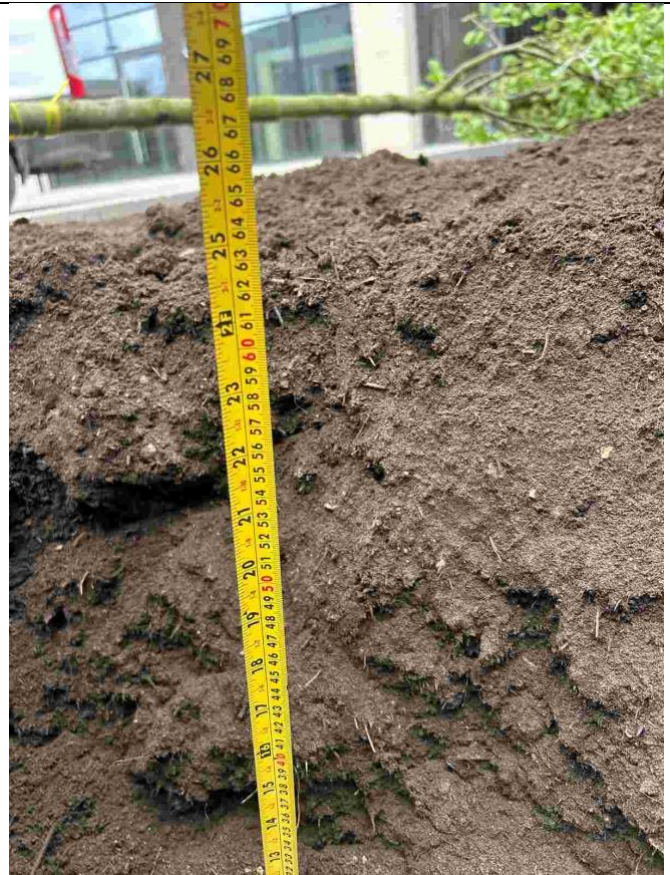
60cm Depth of Topsoil (Block C – Example)
