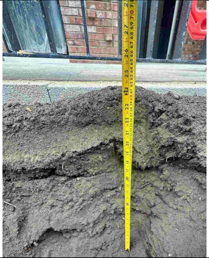
Example of 60cm topsoil thickness (Block B)
