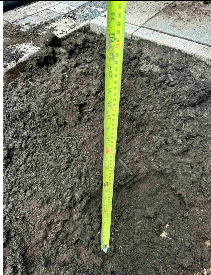
Example of 60cm topsoil thickness (Blocks A and D)
