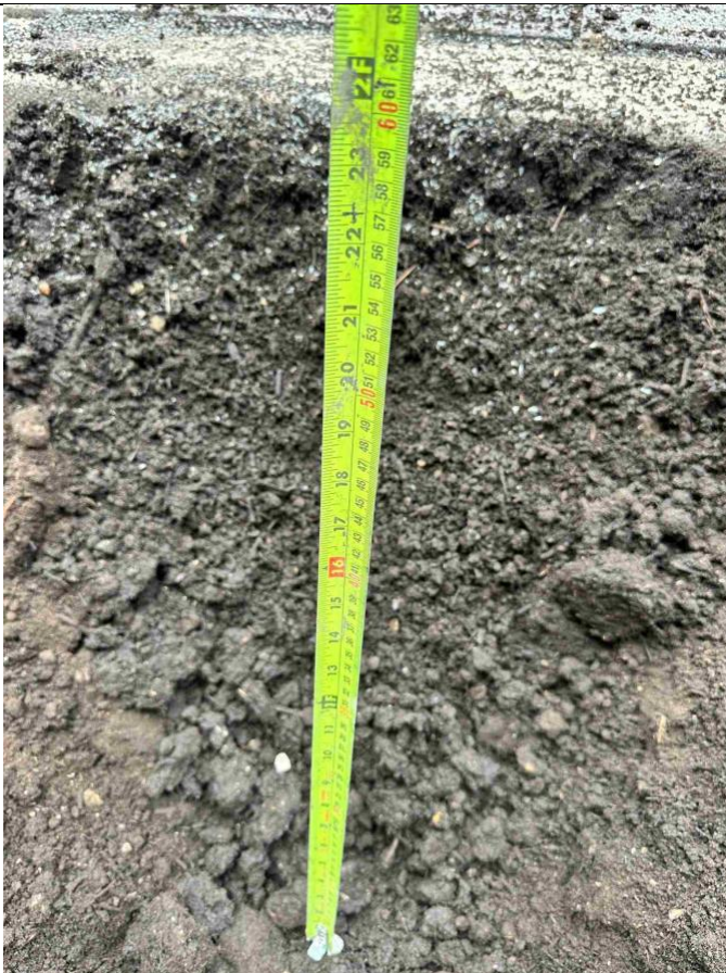
Example of 60cm topsoil thickness (Blocks A and D)
