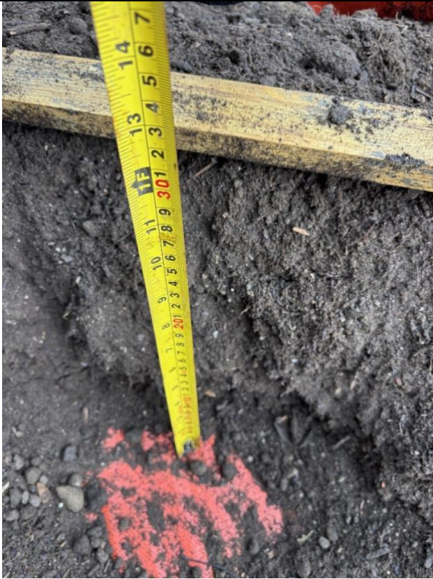
Reduced thickness example within asset protection in Block F
