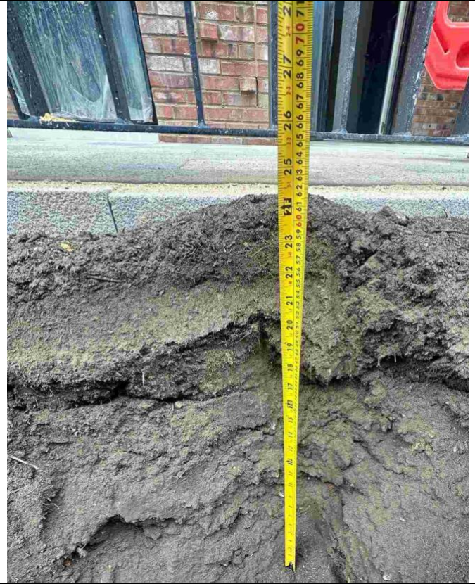
Example of 60cm topsoil thickness (Block B)
