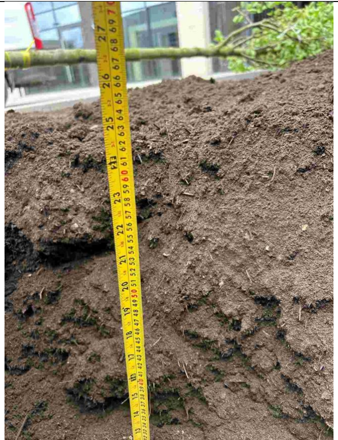
60cm Depth of Topsoil (Block C – Example)
