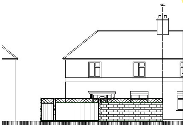
Proposed East Elevation Scale 1:100
