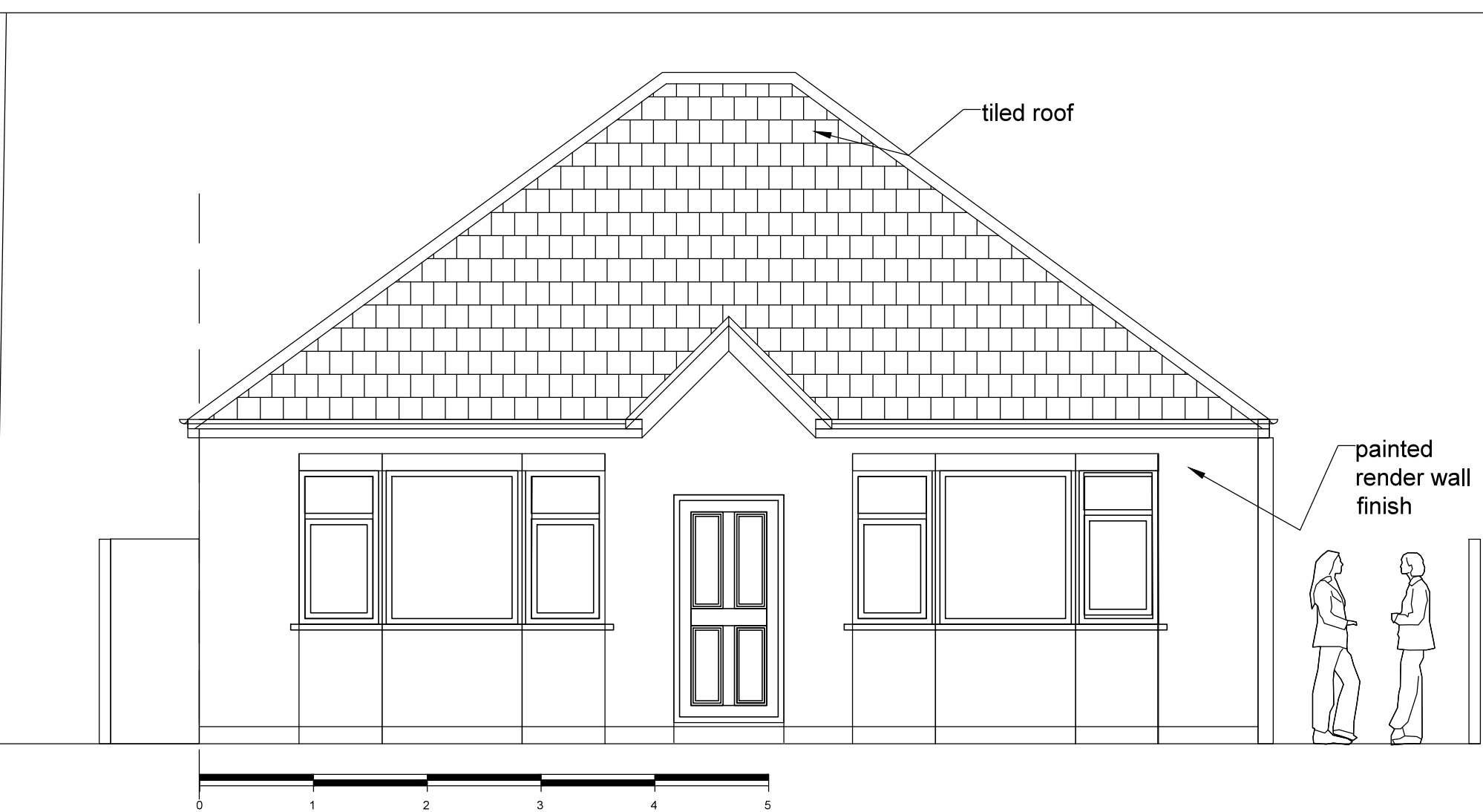
1 FRONT ELEVATION - south west existing - scale 1:50
