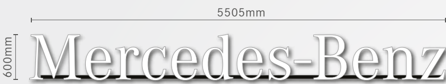
Item A - 360 1no. Set individual white internally illuminated letters with black runner bars. Dimension for situation on buildings columns. Scale 1:50
