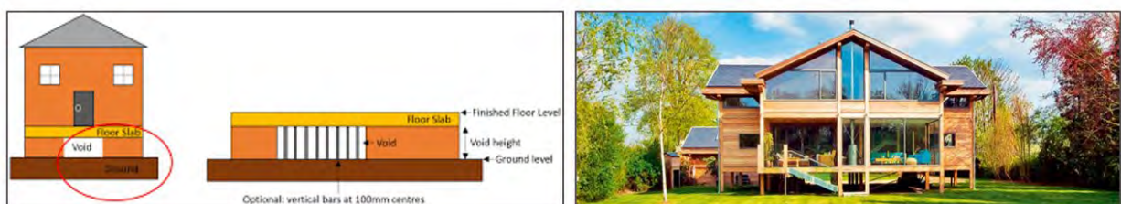
Figure 5. Schematic of theory behind the use of voids for floodplain storage
