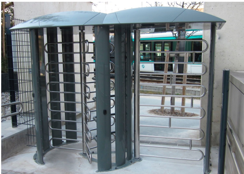
Image to show example of security pedestrian turnstile with wheelchair access pass gate
