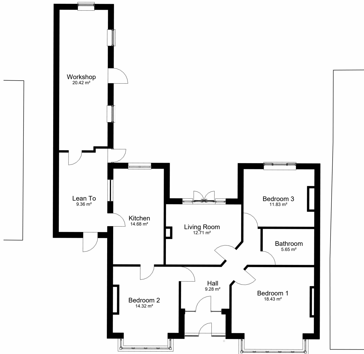
Existing Ground Floor Level 1 : 100
