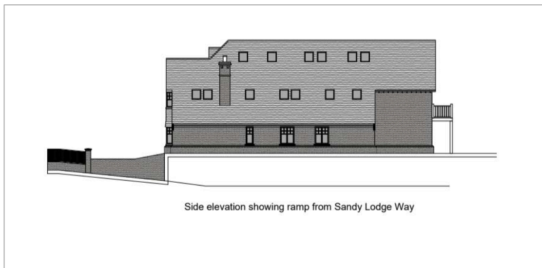
Figure 18: Side elevation showing ramp to basement parking
