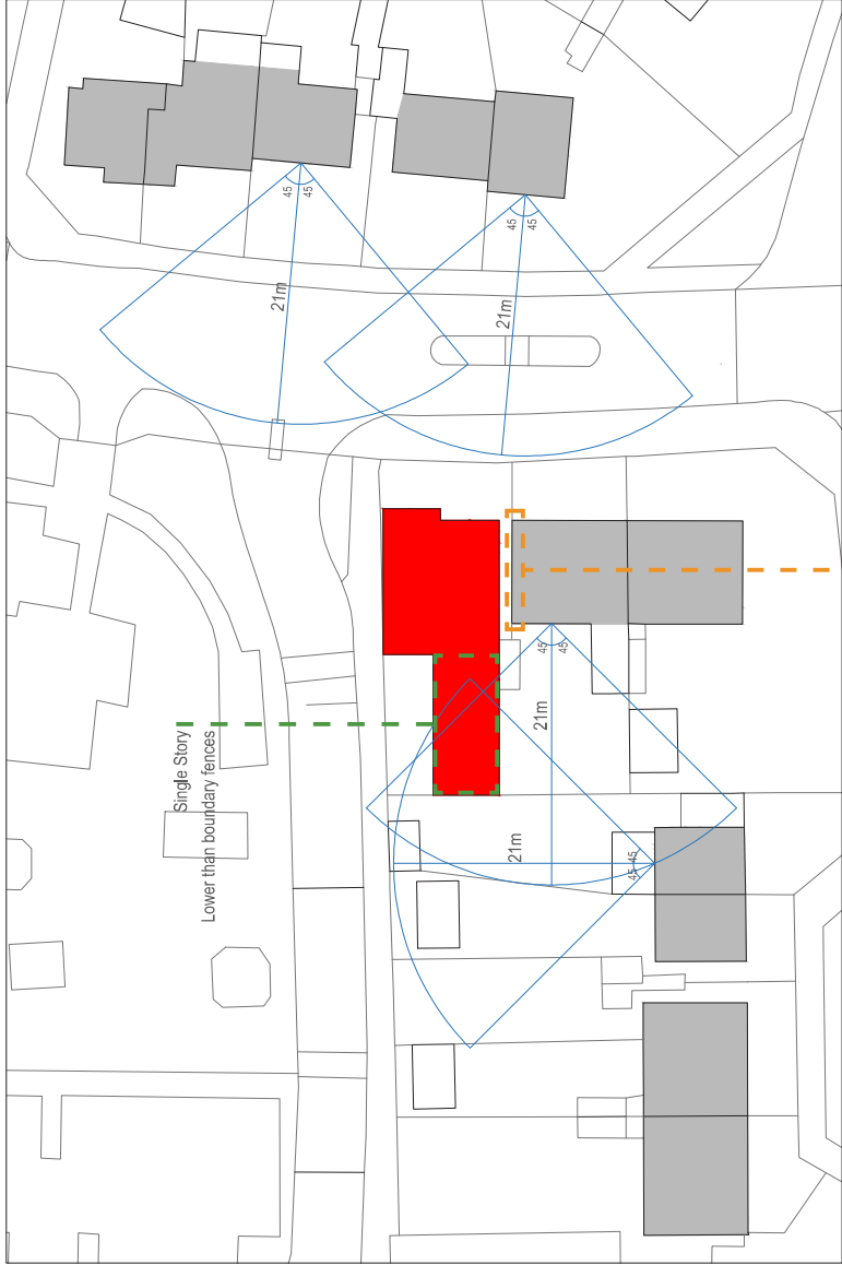
Site Plan showing 45 Degree rule
