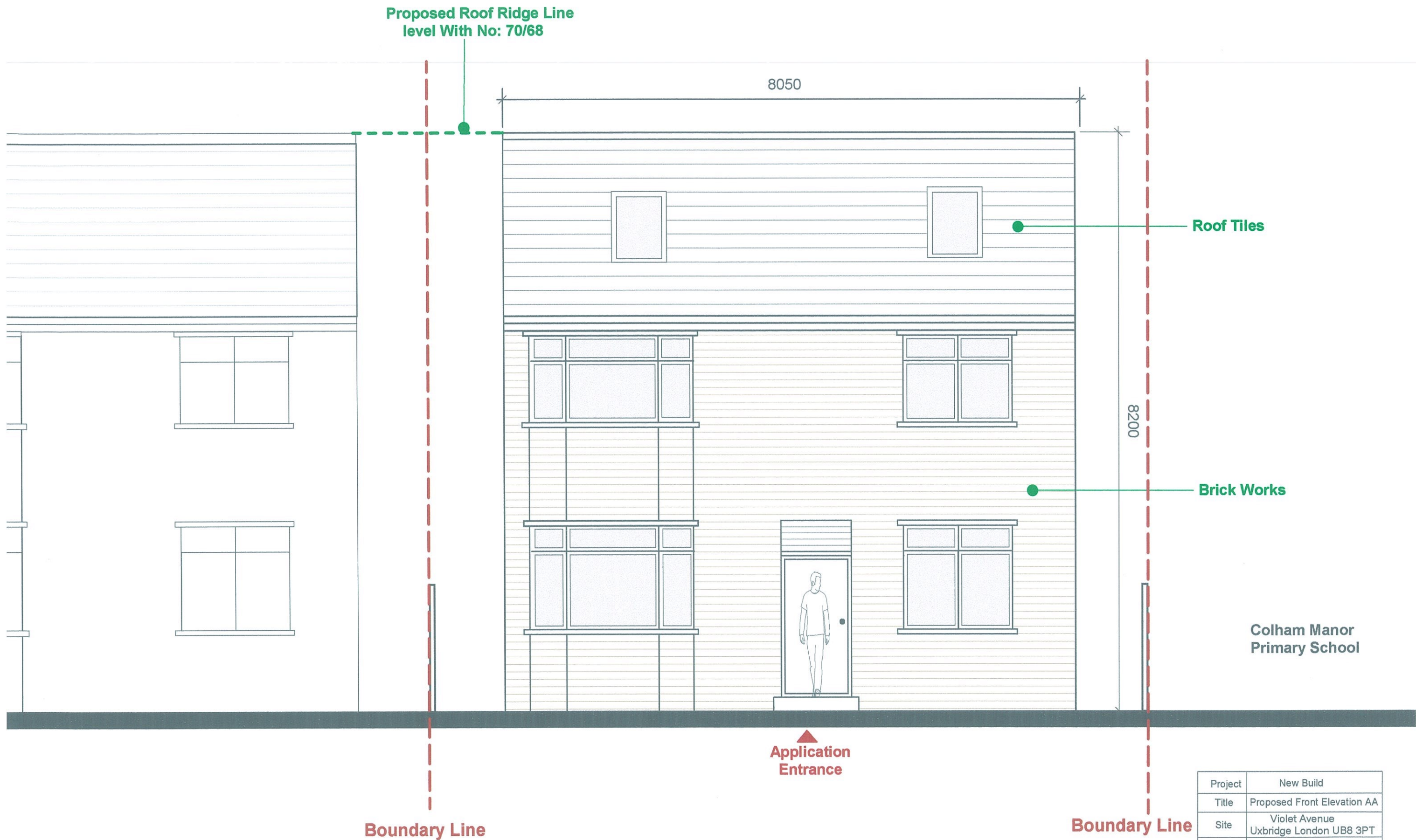
Proposed Front Elevation AA Scale 1:50 @ A3 (New Build)
