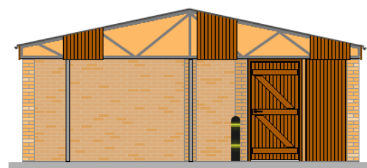
North Elevation (Some timber gable cladding removed to show steel truss frame)
