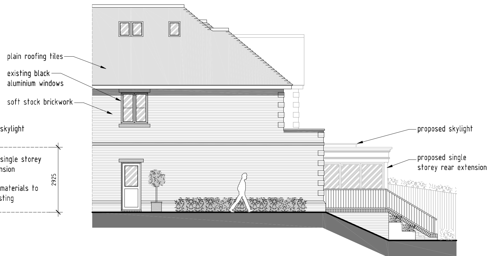
PROPOSED SIDE ELEVATION SCALE 1:100
