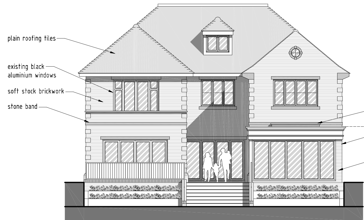
PROPOSED REAR ELEVATION SCALE 1:100
