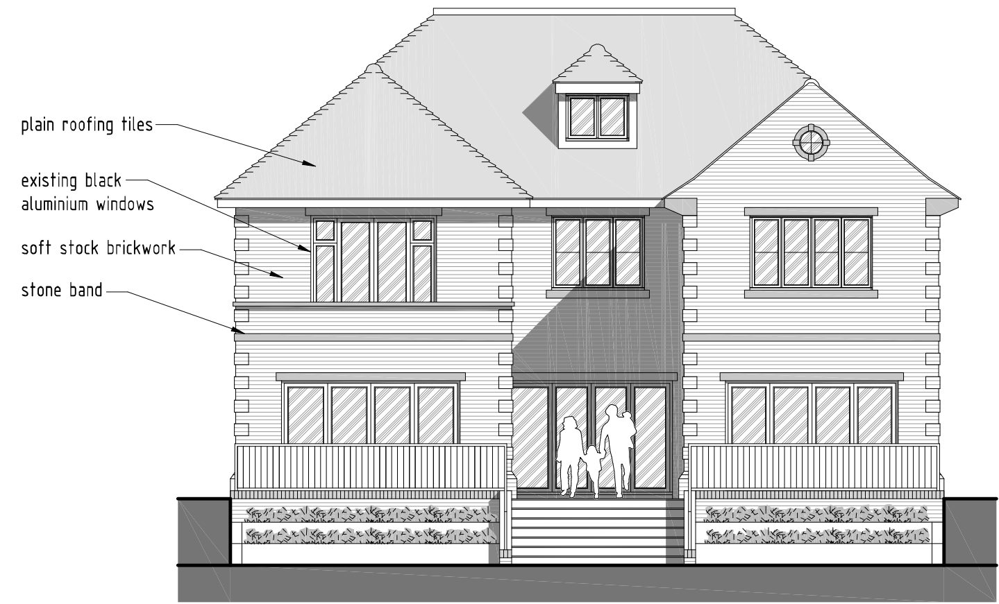
EXISTING REAR ELEVATION SCALE 1:100
