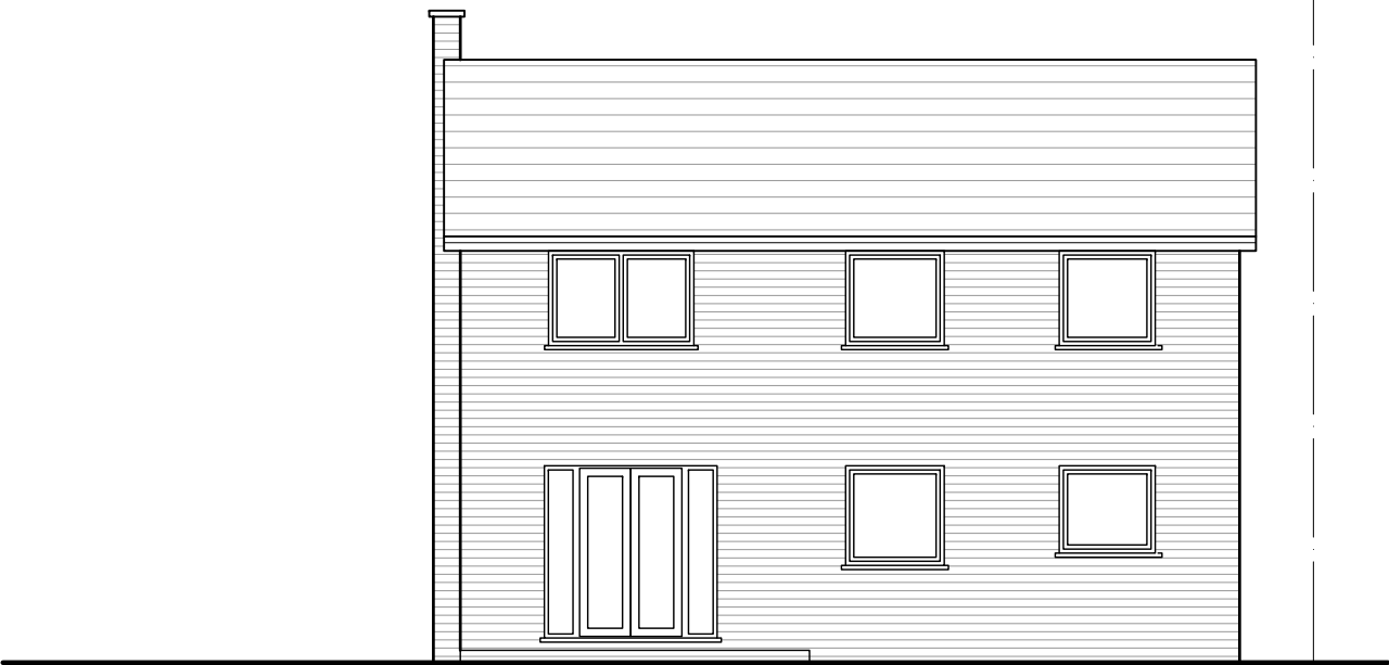
EXISTING REAR EAST ELEVATION
