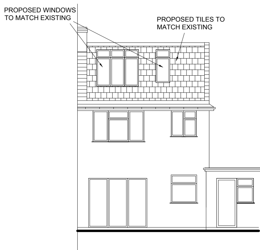
PROPOSED REAR ELEVATION Scale 1:100
