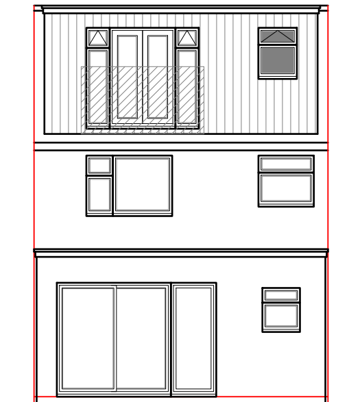
PROPOSED REAR ELEVATION 1:100
