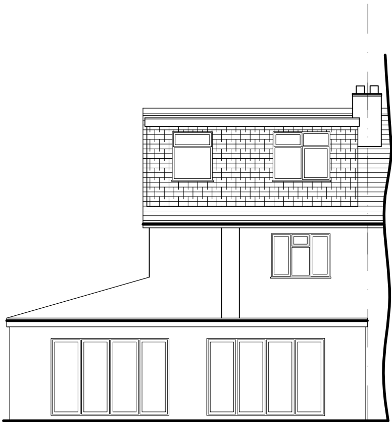
PROPOSED REAR ELEVATION (1:100)
