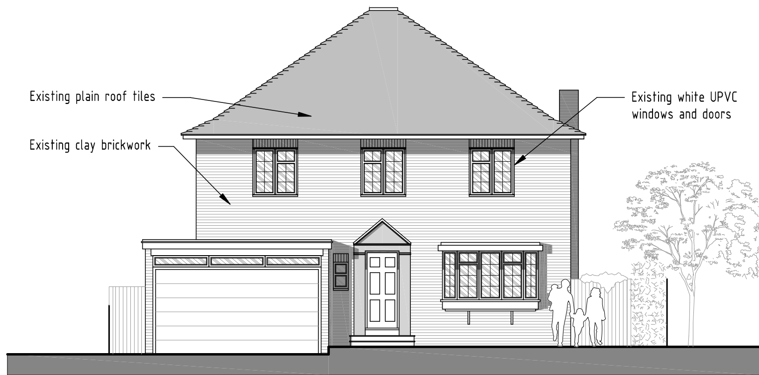
EXISTING FRONT ELEVATION
