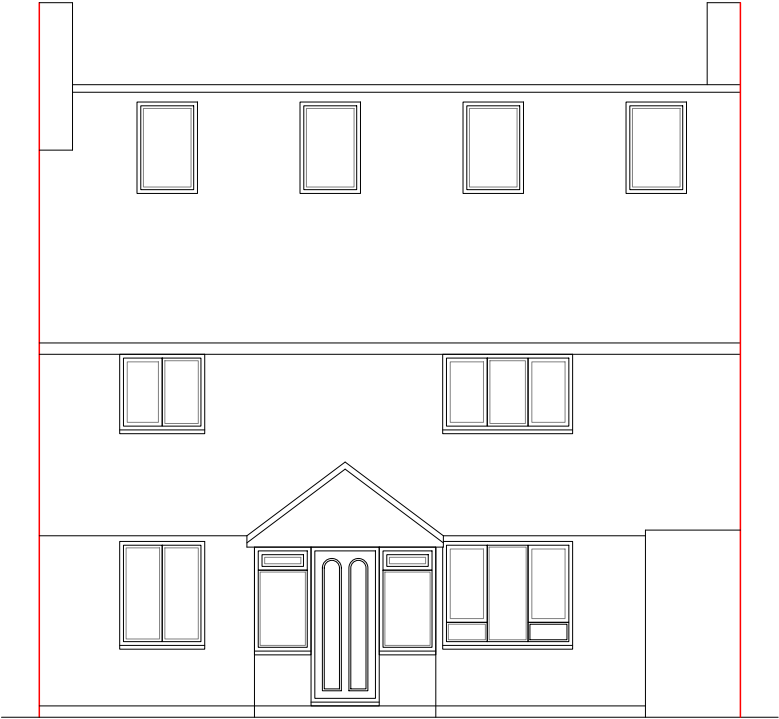
EXISTING FRONT ELEVATION 1:100
