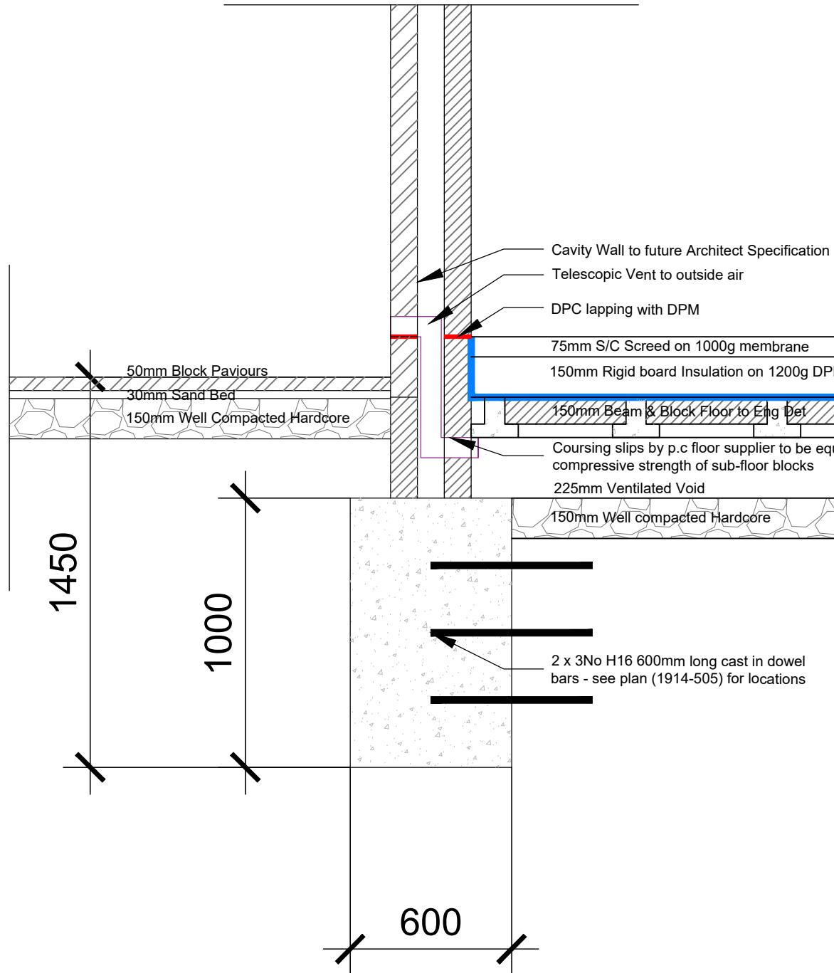
Foundations shown on this drawing are designed for a ground bearing capacity of 100kN/m<sup>2</sup>. If ground condition is found to be less than this capacity, foundations design to be amended by suitably qualified Structural Engineer.
