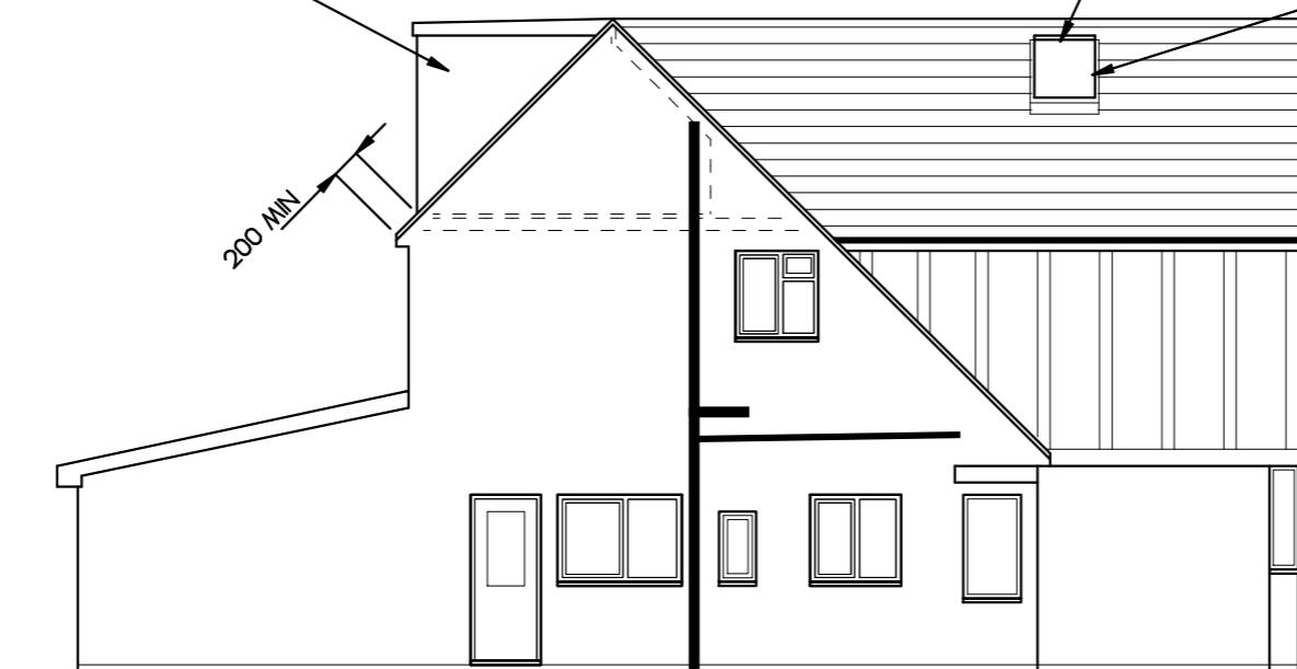
ALL ROOFLIGHTS MUST NOT PROTRUDE MORE THAN 150mm BEYOND THE PLANE OF THE SLOPE OF THE ORIGINAL ROOF
