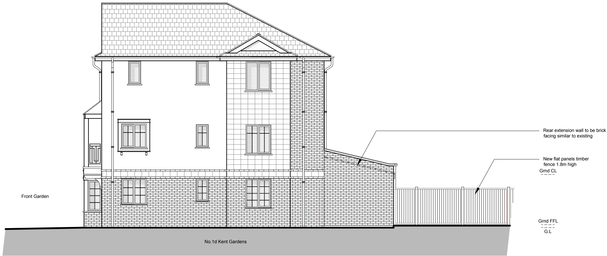
Side Elevation As Proposed - Scale 1:100
