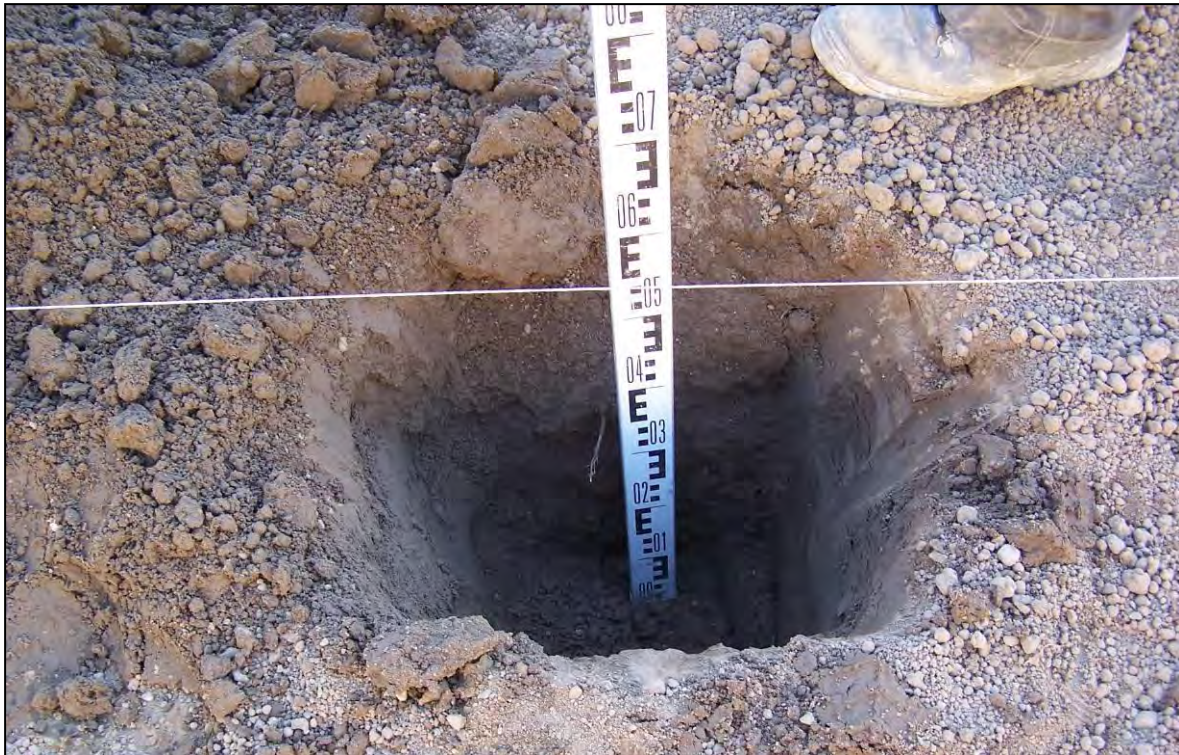
Plate 2 Clean Cover Verification Hand-Dug Pit
