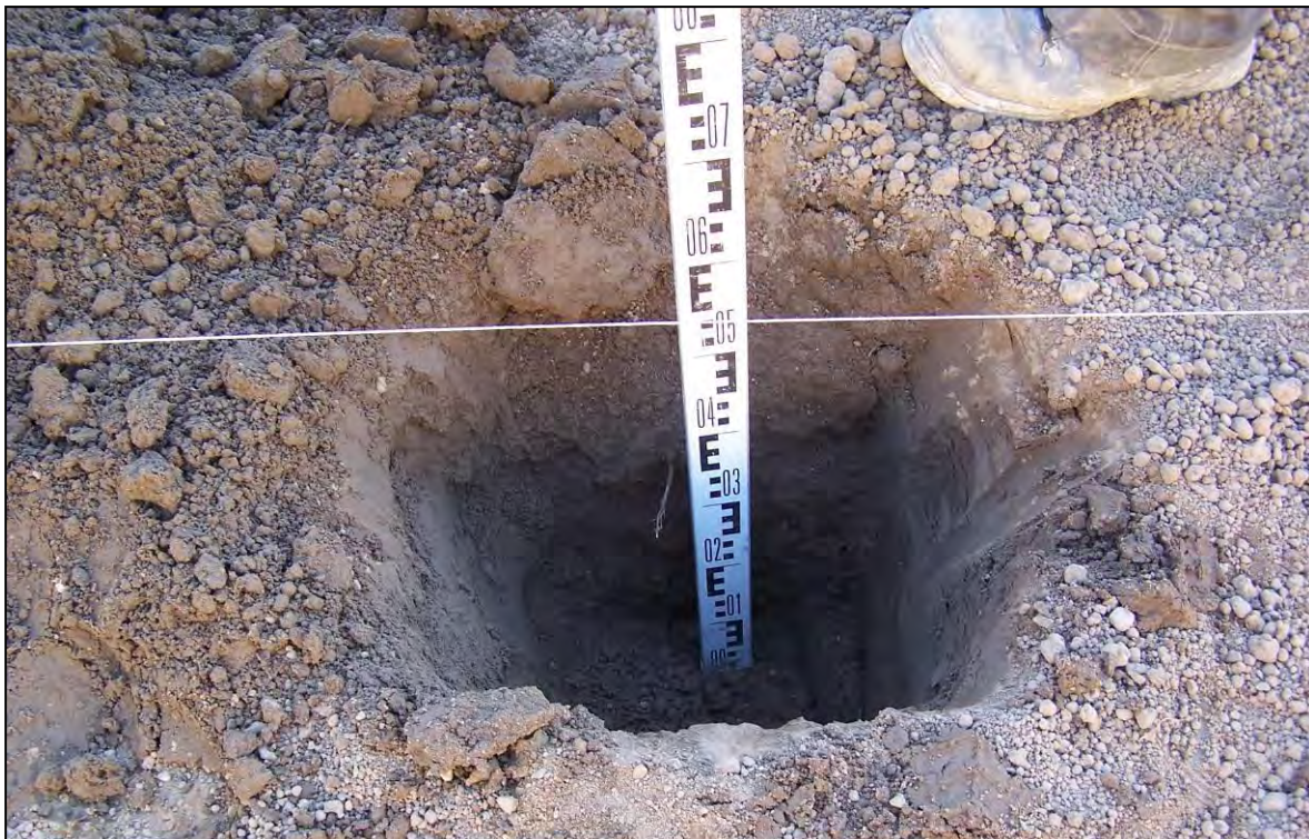
Plate 2 Clean Cover Verification Hand-Dug Pit
