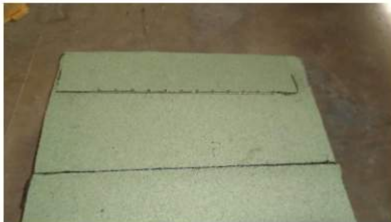
Figure 2: Green granular coating with metal spikes
