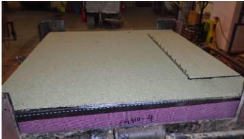
Figure 4: Test specimen before application of sedum layer and side boards, showing retention strip
