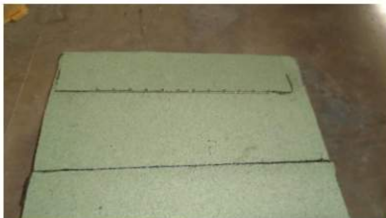
Figure 2: Green granular coating with metal spikes
