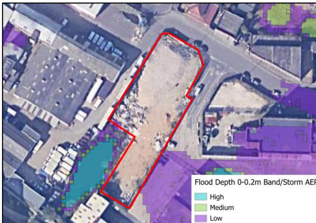
Figure 2 - RoFSW Flood Depths
