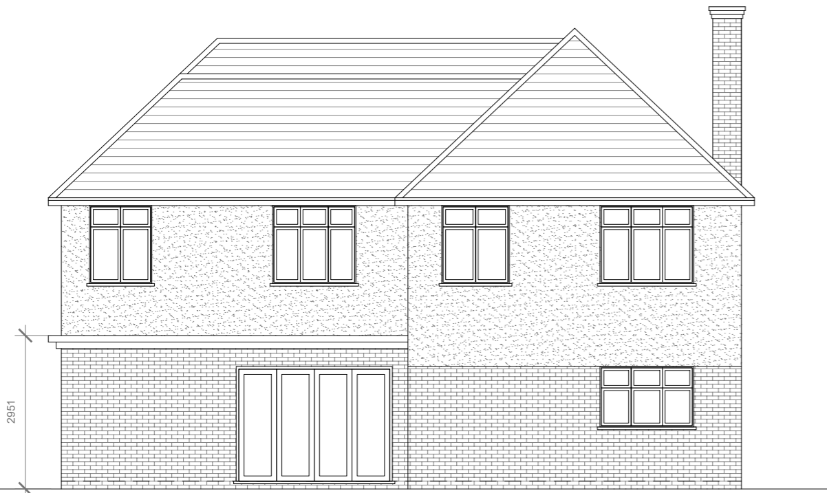
Proposed Rear Elevation Scale 1:100
