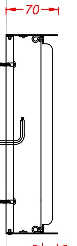
Built-up letters have 1.2mm descaled stainless steel faces and returns which are finished black-grey RAL 7021 and the faces are set back within the returns for an open-trough appearance. Fret cut lines in the faces are fitted with bullnosed 15mm opal 030 acrylic. Fitted with low energy white LEDs for face illumination.
