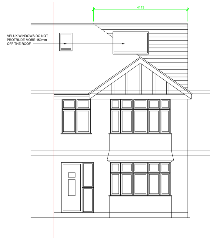
PROPOSED FRONT ELEVATION Scale 1:100
