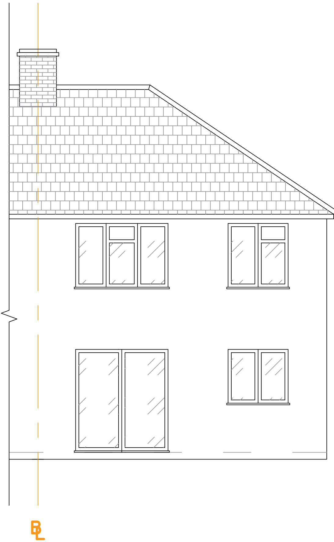
EXISTING REAR ELEVATION SCALE 1:50
