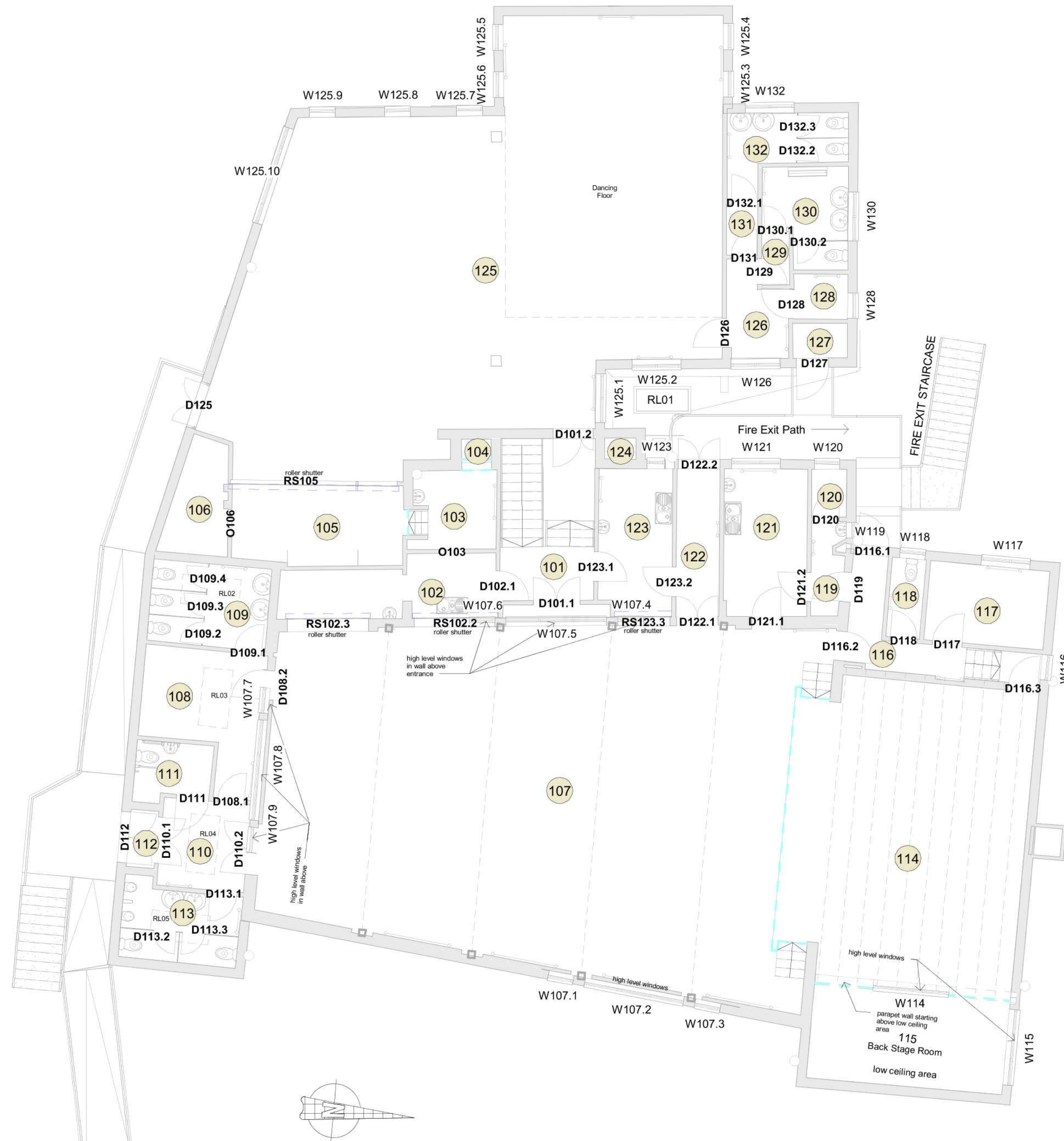
01 Existing - First Floor - Door & Window Location Plan 1 : 100
