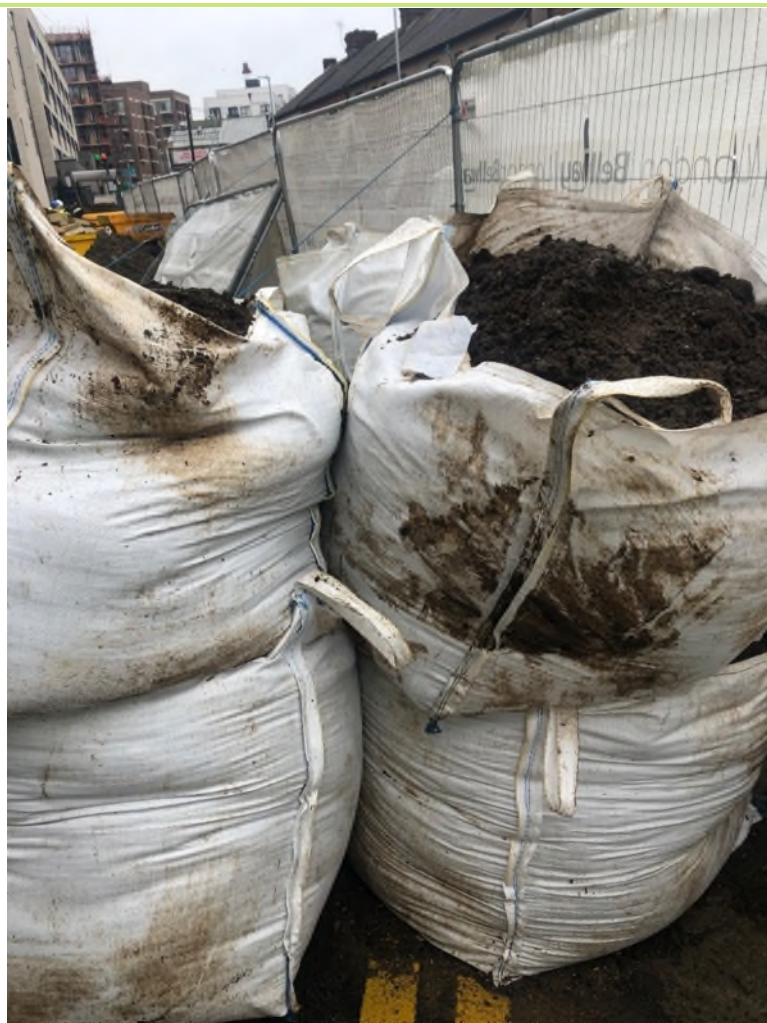
Plate 16: Topsoil bulk bags 1 and 2 from which environmental samples were taken (Taken by LEAP Engineer).
