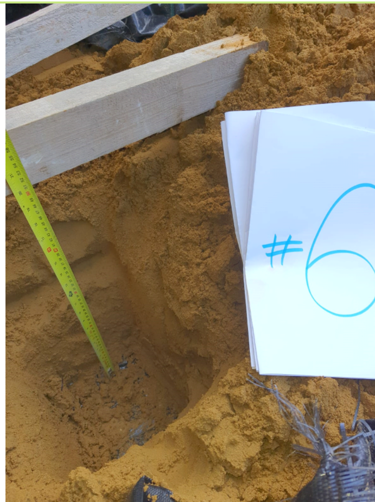
Plate 13: Plot 6 hand dug pit with thickness of subsoils indicated (Provided by Bellway)
