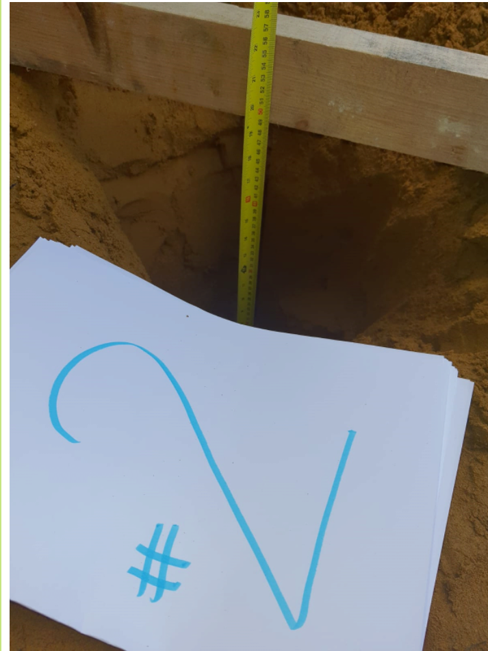
Plate 9: Plot 2 hand dug pit with thickness of subsoils indicated (Provided by Bellway)
