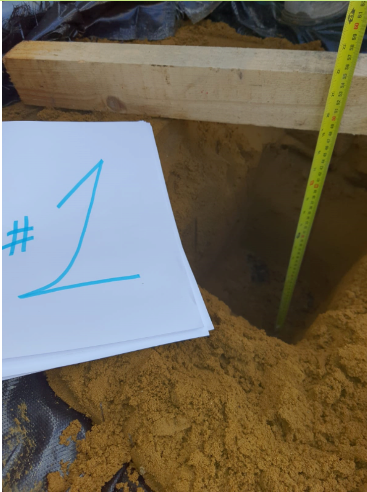
Plate 8: Plot 1 hand dug pit with thickness of subsoils indicated (Provided by Bellway)
