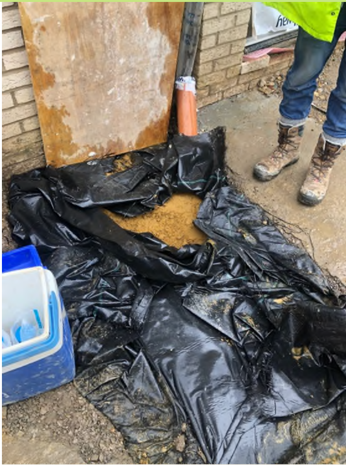
Plate 7: Plot 4 with geotextile wrap around subsoil within shrub planting area from which an environmental sample was taken (Taken by LEAP Engineer).
