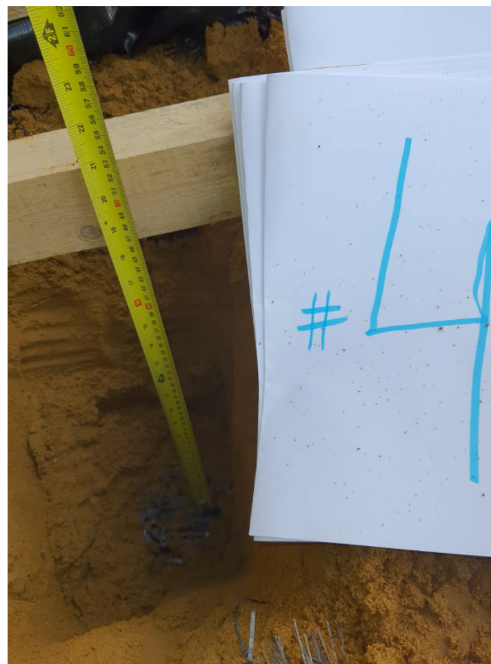
Plate 11: Plot 4 hand dug pit with thickness of subsoils indicated (Provided by Bellway)
