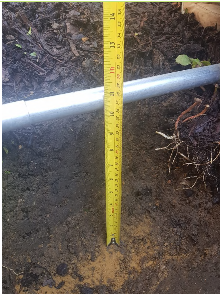
Plate 15: Plot 6 with thickness of topsoil indicated (provided by Bellway).
