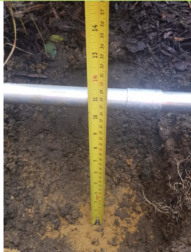
Plate 12: Plot 4 with thickness of topsoil indicated (provided by Bellway).
