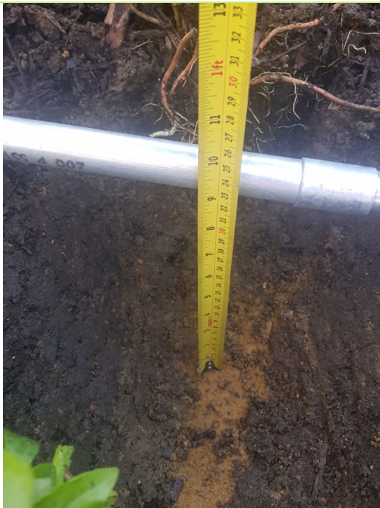
Plate 17: Plot 7 with thickness of topsoil indicated (provided by Bellway).
