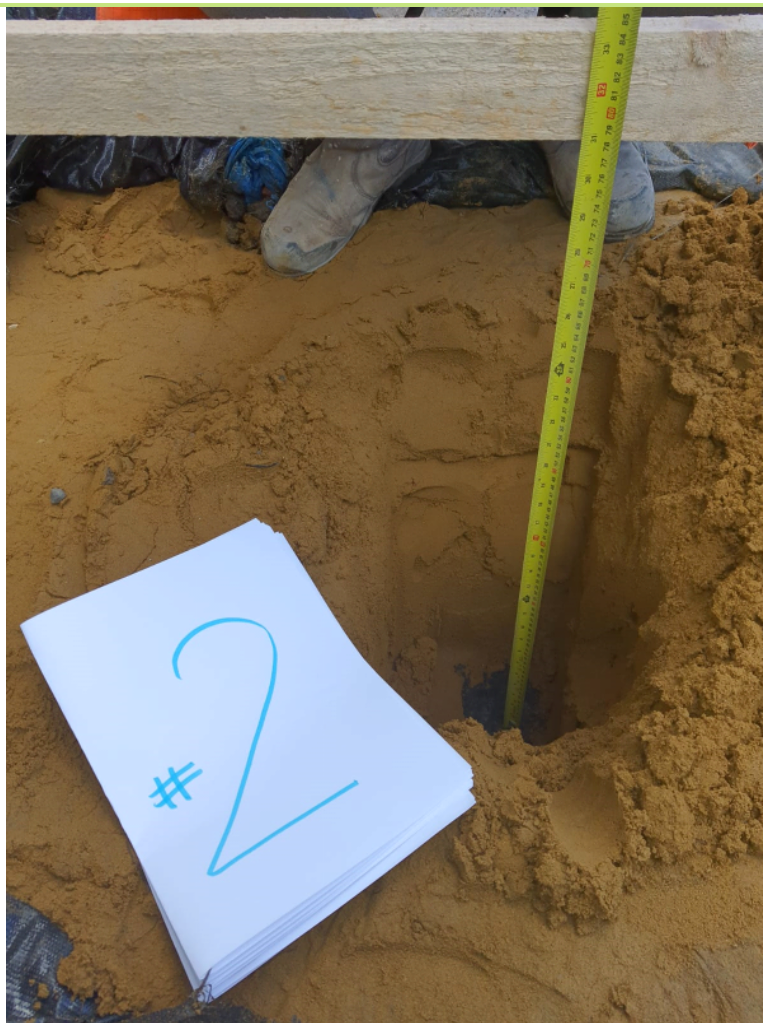
Plate 5: Plot 2 hand dug with geomembrane visible (Provided by Bellway).
