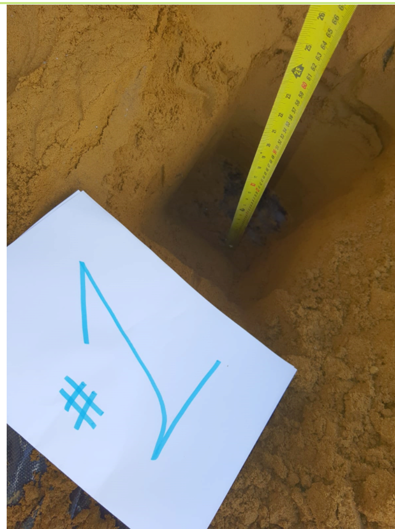
Plate 2: Plot 1 hand dug with geomembrane visible (Provided by Bellway).
