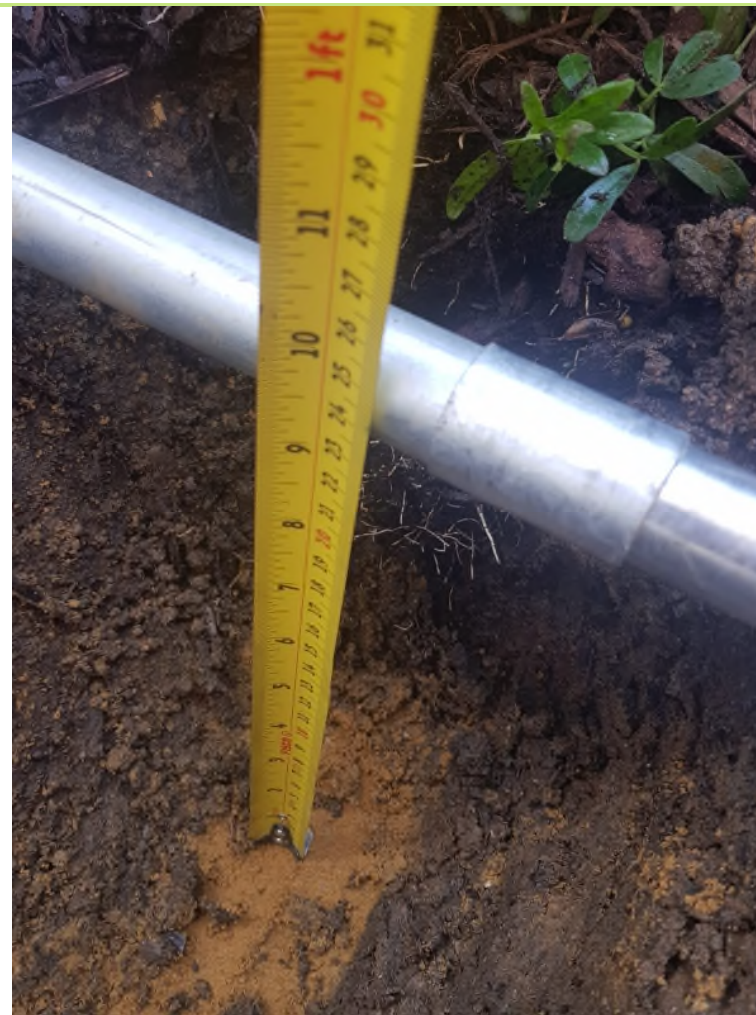
Plate 6: Plot 2 hand dug pit with thickness of topsoil indicated (Provided by Bellway).
