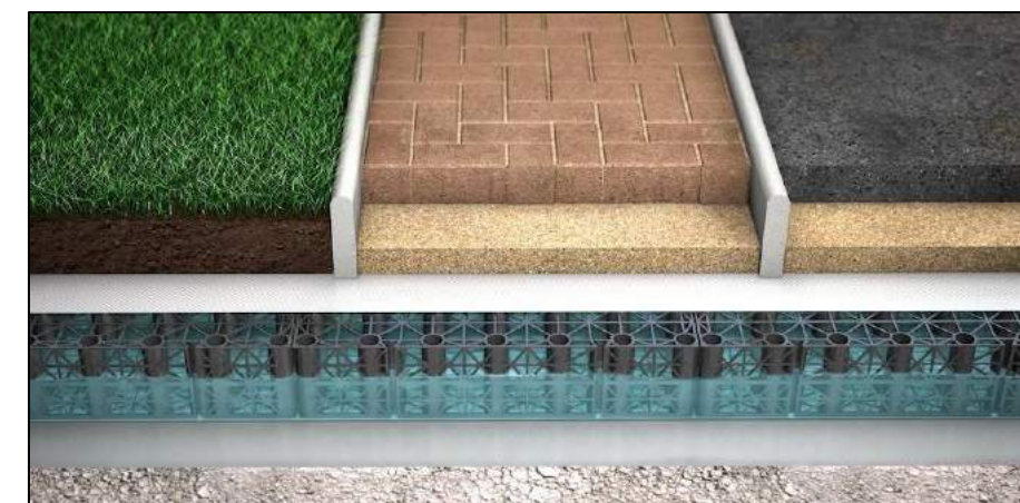
Figure 3-1 Permeable paving with geo-cellular sub-base
