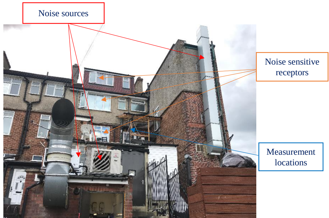
Figure 3: Measurement set-up, noise sensitive receptors, noise sources at the site and showing measurements position at the rear of the site.
